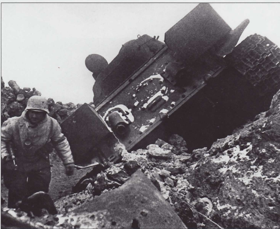
A 9mm MP40 machine pistol-armed scout makes his way past a mired T-34/76. The boxy objects over the rear fenders are auxiliary fuel tanks that would normally be discarded in combat. German troops would habitually drain the much needed fuel from knocked out and abandoned vehicles.
