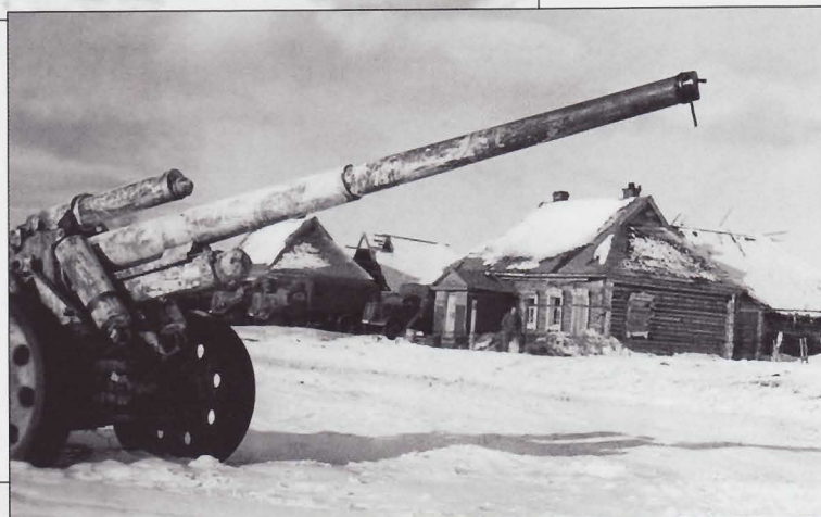
A 10cm K18 Kanone used for counterbattery fire. Its actual caliber was 10.5cm. At 19,075 meters it was the longest ranged piece possessed by the infantry division. Most divisions had one battery in the heavy artillery battalion. Those not provided a 10cm battery received an additional battery of 15cm howitzers.
