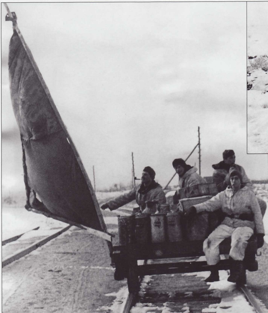
Transport came in many forms. Here a truck (set of railroad car wheels), probably from a destroyed boxcar, has had a platform built on it and is propelled by a sail harnessing the wind blowing across the steppes. The inventive Landser railroaders are delivering soup and other rations in milk cans and insulated containers as well as ammunition to frontline positions.
