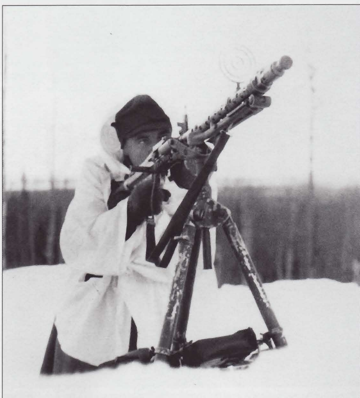
A 7.92mm MG34 machine gun set up on a Dreifuss 34 anti-aircraft tripod and fitted with an anti-aircraft ring sight and a 50-round belt drum magazine. Headquarters and support units possessed a small number of machine guns for ground and air defense. Each artillery battery had two such machine guns, each with a dedicated gunner. Additional crewmen were detailed from the battery.
