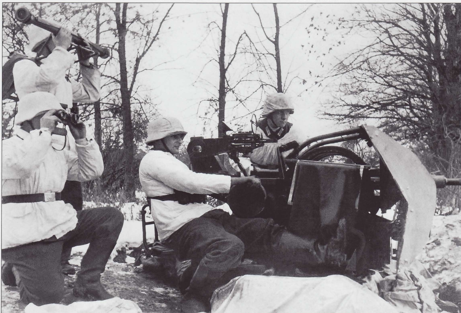
A Heer 2cm Flak 38 anti-aircraft gun crew sights on a target. With a 450 round per minute rate of fire with high-explosive and firing armor-piercing rounds the 2cm Flak could inflict considerable damage on troops, light armored vehicles, and weapon positions. Due to the necessity of changing its 20-round magazine its practical rate of fire was 220 rounds per minute. Nonetheless it proved a valuable weapon for defending sectors thinly held by infantrymen. In the foreground can be seen its white camouflaging/protective tarpaulin.
