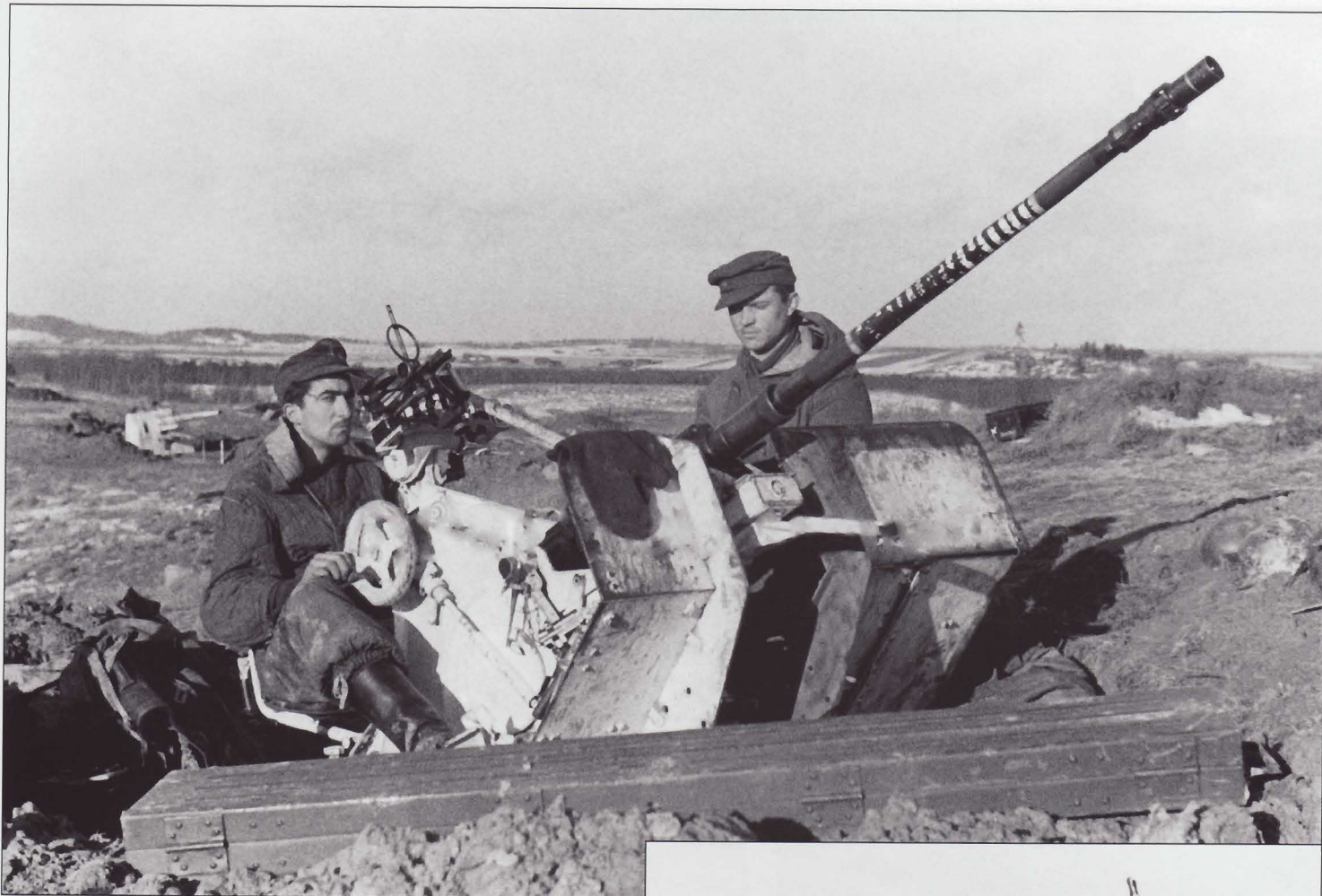
The same gun crewmen run through a test after cleaning the gun to ensure it operates perfectly. The long case to the front contains two spare barrels. Note the 18 kill rings (Abschussringe), partly worn off on the lower knuckled handgrip band. Over the gunner's shoulder can be seen one of the 8.8cm guns that the light Flak is protecting.
