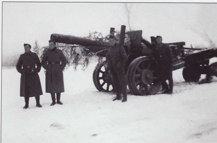
A great deal of Soviet armament was captured and put into German service, either augmenting or substituting for equivalent German equipment. Here a Soviet 152mm ML-20 (M1937) gun-howitzer serves in a divisional heavy artillery battalion. The Germans called it a 15.2cm K.H. 433/1(r) cannon-howitzer. It was almost 1,000 kilograms heavier than the German 15cm s.FH18, but it offered almost 5,000 meters more range. Soviet artillery usually outranged their German counterparts. The Germans also used the 152mm in the coastal defense role being deployed as such in France. Horse- or tractor-drawn pieces were fitted with spoked wheels, but truck-towed weapons had pneumatic tires.
