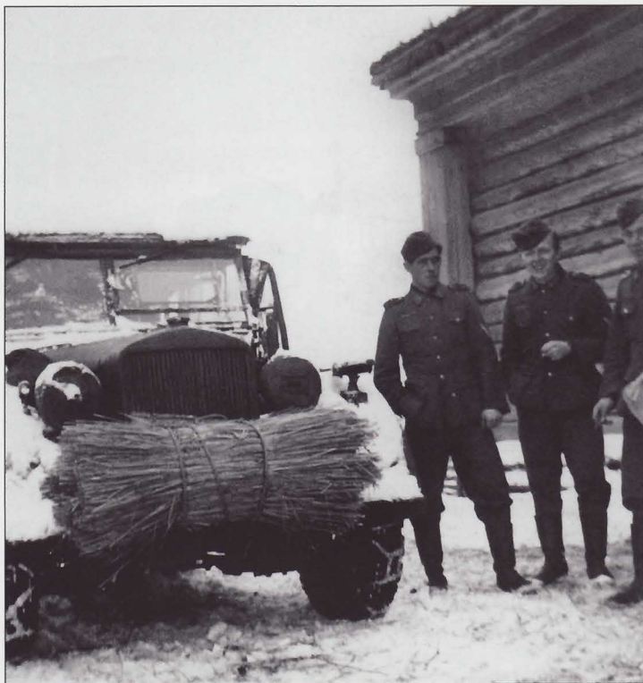
Bundles of reeds were sometimes fastened on trucks to serve as matting if they became stuck in loose snow. The same technique was used to combat the spring and autumn mud.
