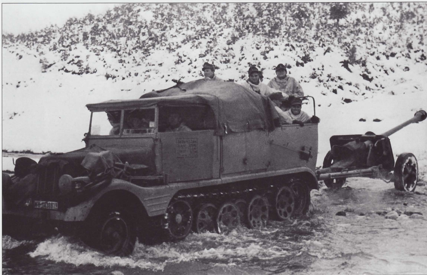
The crew of a 7.5cm Pak 40 antitank gun crosses a mountain stream aboard a 3-ton Sd.Kfz.11 light halftrack (leichter Zugkraftwagen). The 7.5cm Pak was mainly a divisional antitank gun, but some were assigned to regimental antitank companies. The canvas troop compartment cover provided some comfort, but like any unheated vehicle this one offered a cold ride.
