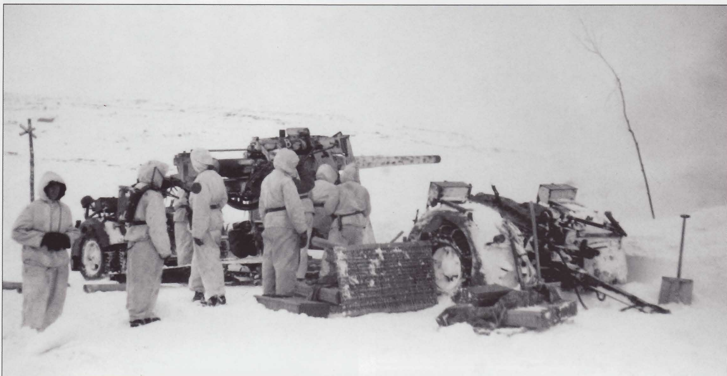
An 8.8cm Flak 18 in full recoil as it fires at a tank at long-range. The "Acht-Acht" could knock out just about any tank at its maximum range, which was beyond the range of most tank guns. This particular gun was designated "B" for Berta. The gun's two limbers (Sonnderanhänger 201) are kept close to speed displacement.
