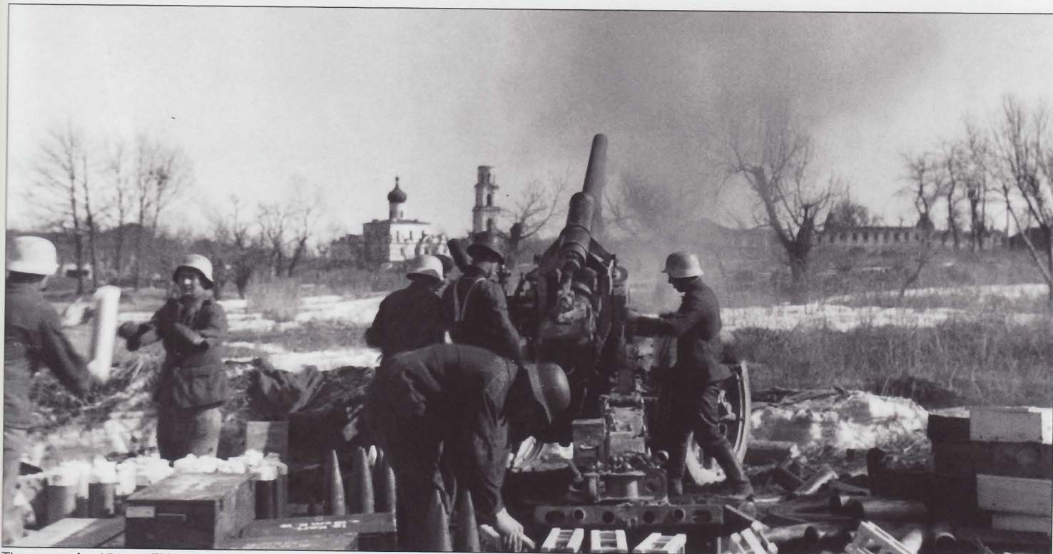
The crew of a 15cm s.FH18 howitzer pumps out rounds. The projectiles were shipped in the wooden frames containers and the cartridge cases in the boxes.
